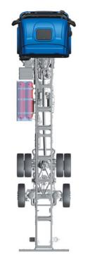
CNG tanks on the left side, available in combination with CNG or LNG tanks on the right side.
